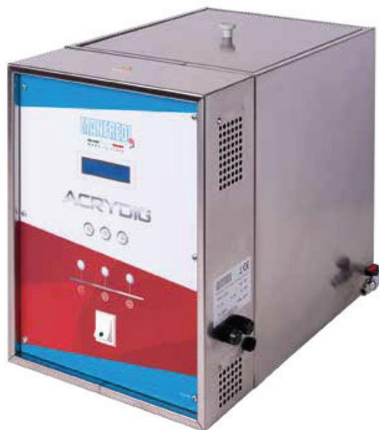
**ACRYDIG polymerizing** units are completely built in stainless steel to guarantee a longlasting life. The special design of the closing lid avoids any dispersion of steam or condensate dripping, thus ensuring the polymerization cycle in a steam saturated atmosphere. The wide opening and the adequate dimensions of the polymerization tank allow a rational accomodation of the flasks.
